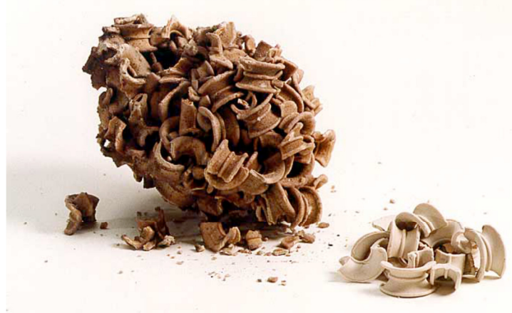
Figure 1 Fused media, left, and new media, right.
